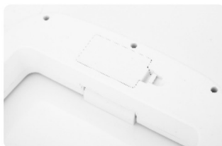
Battery area-back of lid
